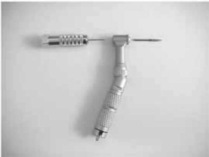
TO REMOVE BUR: PUSH PIN INTO CONTRA ANGLE HEAD, UNTIL BUR FALLS OUT.
