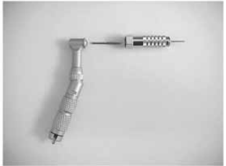
TO INSTALL BUR: INSERT BUR INTO HEAD CAP, USE RUBBER END OF TOOL TO PUSH BUR INTO THE CONTRA ANGLE HEAD.
